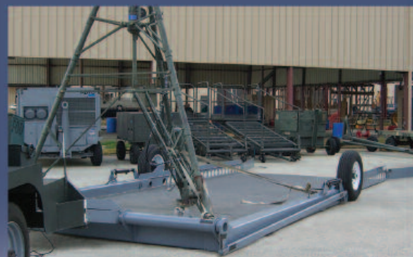
The Wing Jack Trailer is designed for wing jack transportation only.
